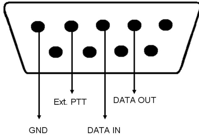
*Note: DATA IN and DATA OUT are used for analog audio in and out; they are not the Rx and Tx data pins for RS-232 communications.*
