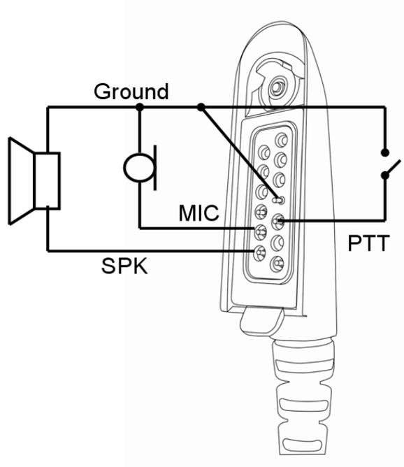
The Radio Terminal Connector should be connected to the above headset as shown below.
