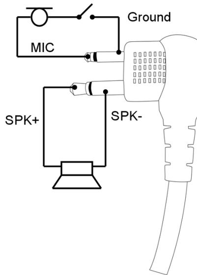
The Radio Terminal Connector should be connected to the above headset as shown below.
